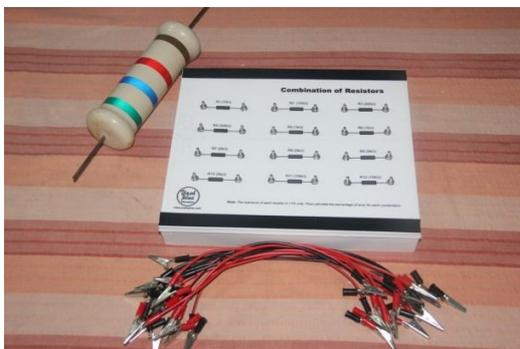
This is the basic kit of doing all types of experiments related to resistors. It can be used for series & parallel combination of resistors, complicated combinations, understanding effective resistance of circuits, current calculations, calculation of wattage (*power dissipation*) of resistors and many more.
